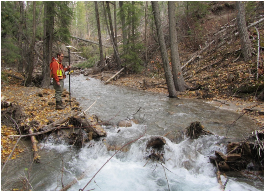
Photo 16. Upstream view of aggradation upstream of a small LWD grade control indicated by the buried roots of the wetted tree on the left bank (photo right); Sta. 4+980(immediately downstream of north-south channel confluence).
